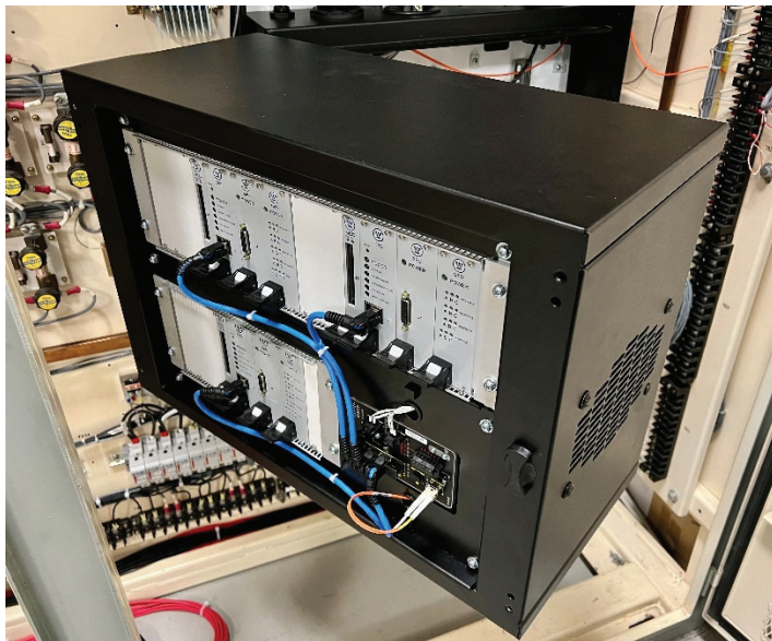
Figure 1-2 –ARCH control assembly is designed for ease of maintenance and installation, with the rear of the electronics assembly accessible.
