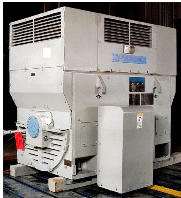
New safety-related medium-voltage motor
