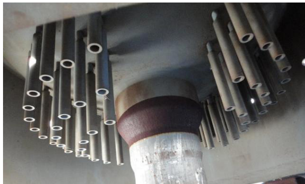
Westinghouse pressurizer lower head mock-up
