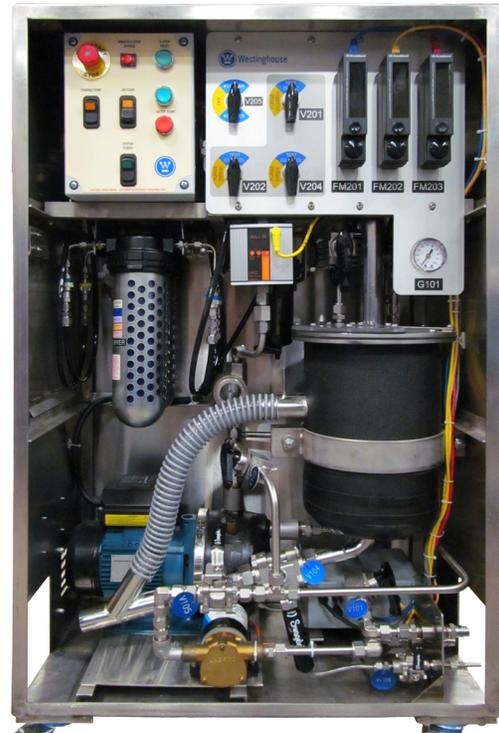
Upgraded TELESCOPE Sipping system built for **AP1000** and applicable for use at all U.S. PWR and BWR plants currently using TELESCOPE Sipping fuel inspection
