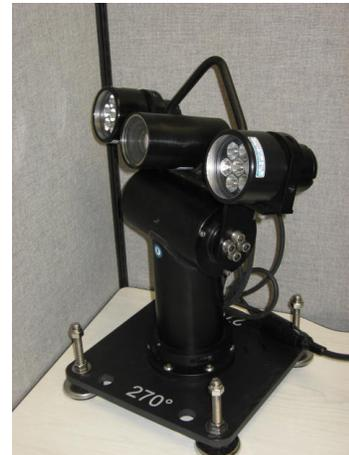
One inspection pod – camera, lights, and pan and tilt on adjustable base
