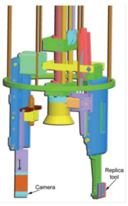
Manipulator for pump housing inspection
