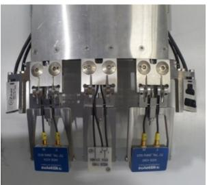
Probe head for 8 mm thick gap for boiler spine inspection CAD design and Actual probe head used
