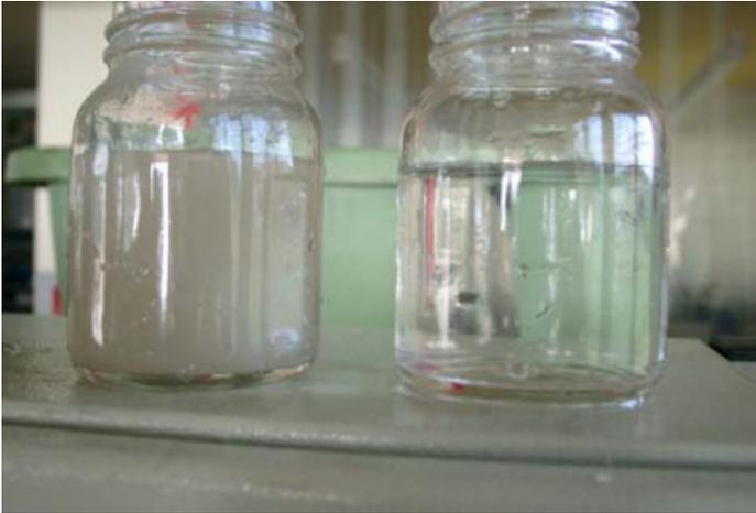
Water sample before and after chamber filtration
