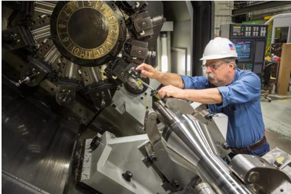
*Core Support Column Machining*
