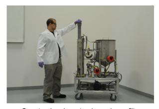
Operator changing out an ion exchange filter
