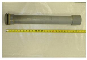
Typical ion exchange filter
