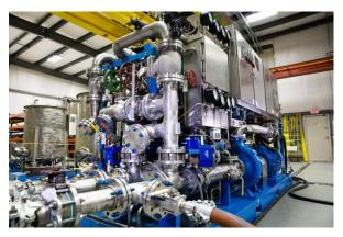
Westinghouse has developed a variety of chemical decontamination processes and skid-mounted equipment, such as that shown above which is capable of processing system volumes greater than 25,000 gallons.
