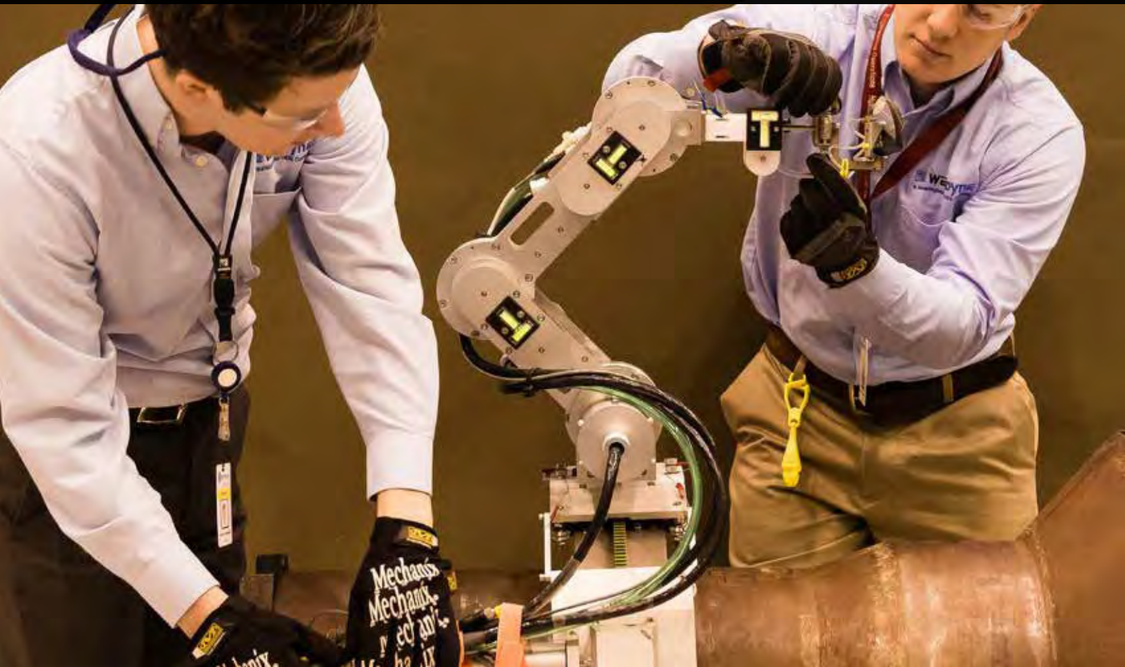
The track-mounted ROSA™-based examination system (T-Rex)
