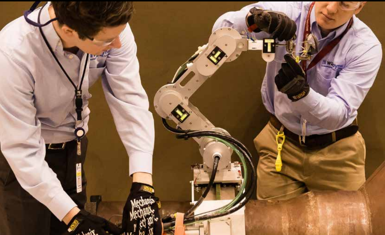
The track-mounted ROSA™-based examination system (T-Rex)
