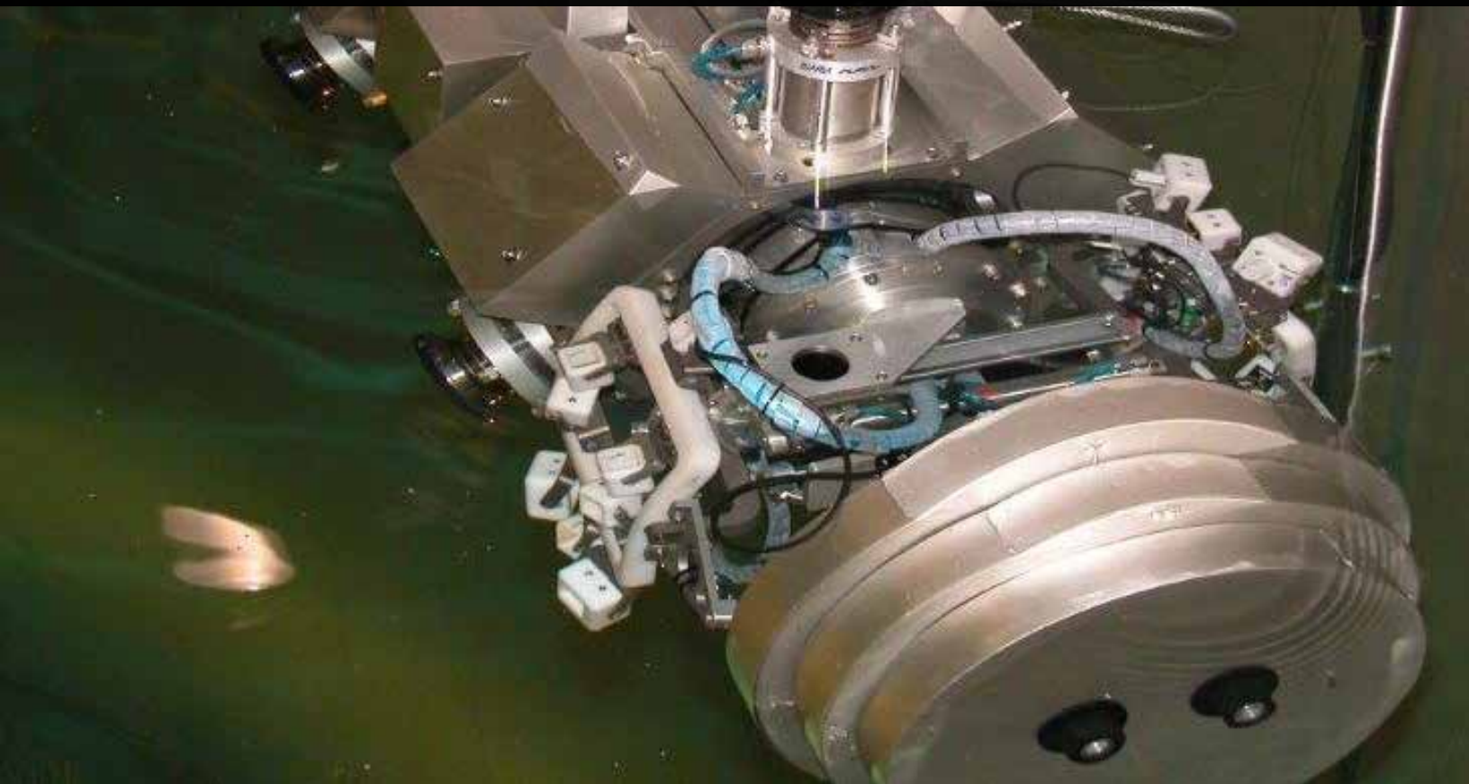
The Westinghouse SQUID (SUPREEM eQuivalent Ultrasonic Inspection Device) scanner
