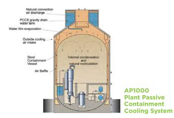
Instead of electrical pumps and back-up diesel generators seen in older, active plants to power containment cooling sprays, the AP1000 plant uses all natural forces. Because the containment cooling water tank is located above containment in the AP1000 plant, gravity provides the only necessary force to deploy the cooling water. Together with condensation and natural circulation, containment cooling is provided without the need for any AC power.
