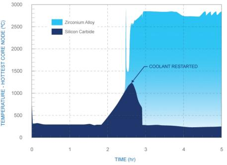
**Fig. 3.** Three Mile Island-2 progress simulation: Silicon-carbide cladding tolerance to heat and steam as compared to that of TMI-2's zirconium alloy cladding.
