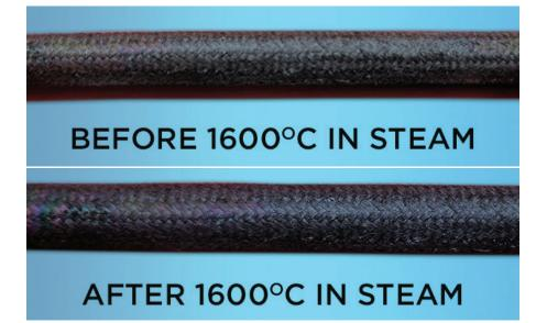
**Fig. 2.** Before and after photos of silicon-carbide cladding severe accident testing at about 1600  $^{\circ}$ C (about 2900  $^{\circ}$ F) for 40 minutes in steam. The cladding exhibited essentially no change or damage.
