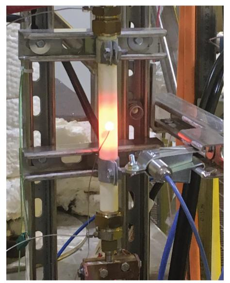
**Fig. 1.** A simulation of a severe accident test of silicon-carbide cladding at about 1600 °C (about 2900 °F) is carried out at Westinghouse's Ultra-high Temperature Test Facility. (Photos and graphs: Westinghouse Electric Company LLC)
