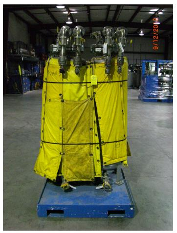
Shielded ion exchange columns on skid
