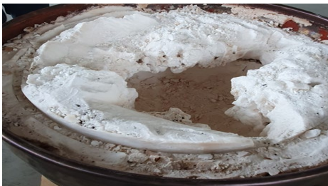
Salt crystals growing beyond the upper edge of the drum into the filling hood and voids.
