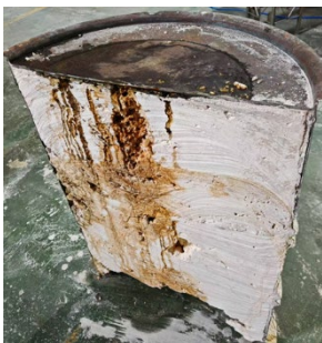
Voids in the center of the final product, and salt encrustation of the filling hood contributed to a limited production Volume Reduction Factor (VRF) of 4.
