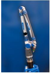
Coordinate measurement machine (articulating arm)
