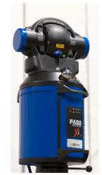
Laser tracking interferometer
